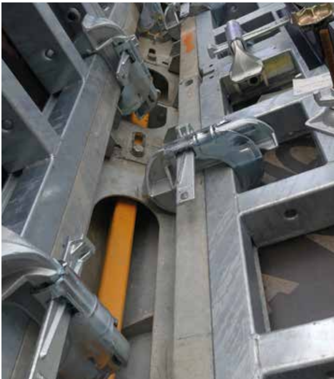
STRIPPING CORNER MAX secure to MEGAFORM panels
